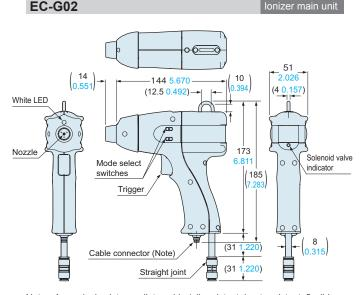
Note: An exclusive intermediate cable (oil-resistant, heat-resistant, flexible type, ø3.7 mm  $\emptyset$ 0.146 in, 2 m 6.562 ft long) is attached.
