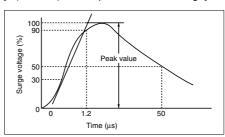
4) Regarding external noise, the values below are considered the noise-resistant voltages. If voltages rise above these values, malfunctions or damage to the internal circuitry may result, so take the necessary precautions.
