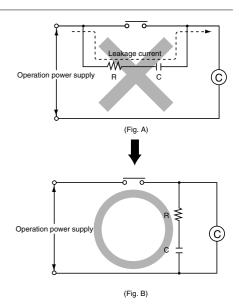
6) Long periods of continuous operation in the count-up completed condition (one month or more) will result in the weakening of the internal electrical components from the generated heat and, therefore, should be avoided. If you do plan to use the unit for such continuous operation, use in conjunction with a relay as shown in the circuit in the diagram below.
