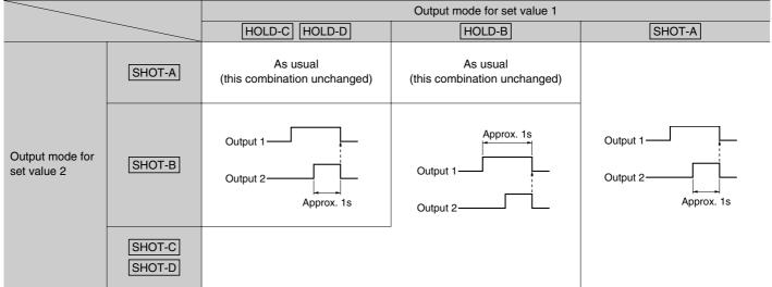
Note: When control output 1 is on, the output mode of Setting 2 (SHOT-A, B, C, D) is also on and output 1 changes as shown in the above table.
