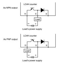
Note: With the LC4H 8-pin type and the LC4H-W, there is no diode between points (8) and (9).
