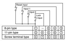
Note: The LC4H-W does not have the lock input (4) 7.
